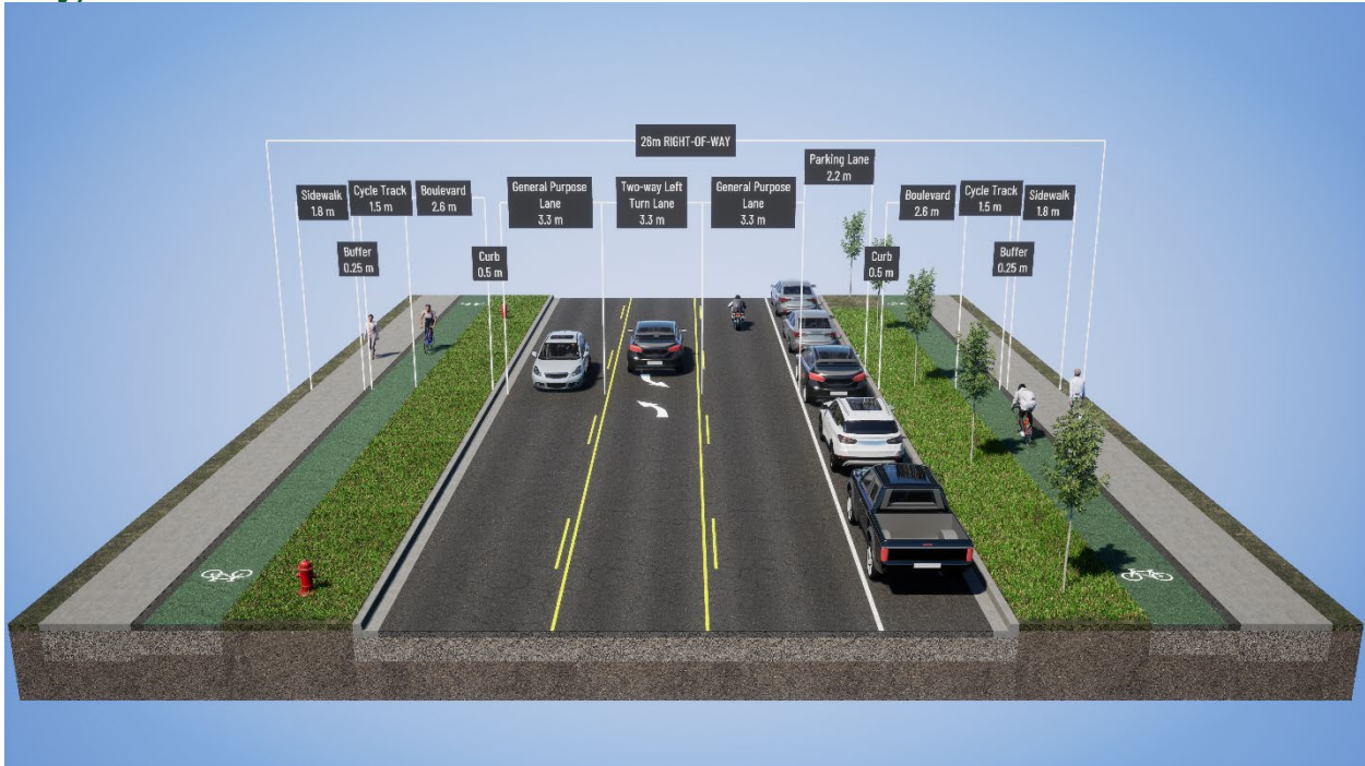
Figure 55. Recommended Major Collector Typical Cross-Section (26m Right-of-Way)
