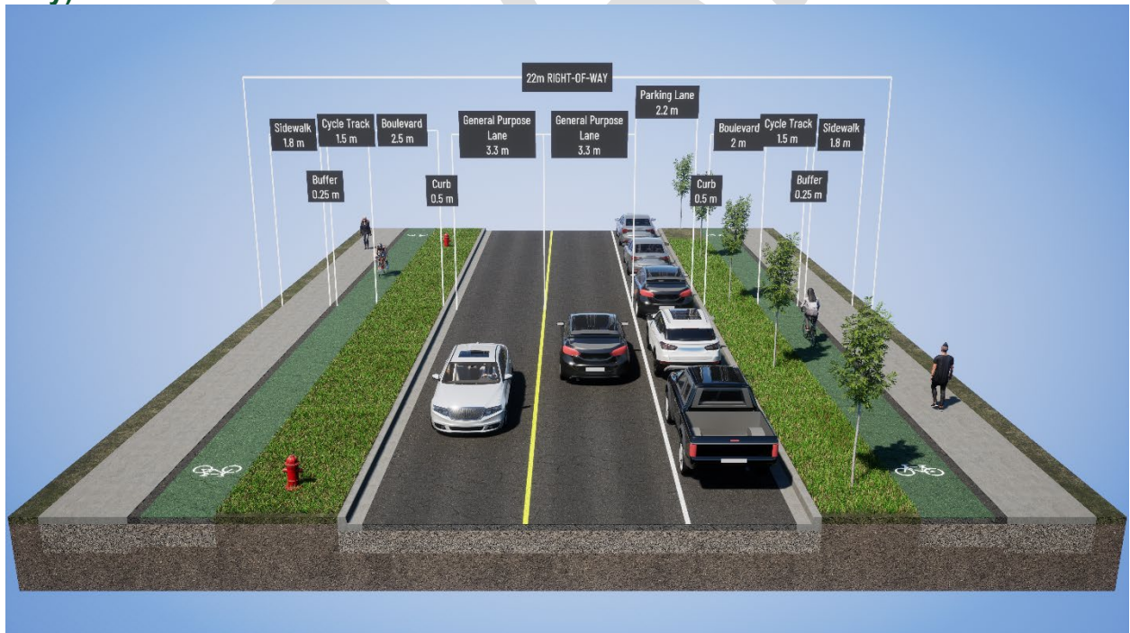
Figure 54. Recommended Minor Collector Typical Cross-Section (22m Right-of-Way)
